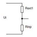
When powered by a certain input voltage, an electric current will flow through both resistors. The current through each resistor is the same (resistors in series). So we can write out the following equation:
