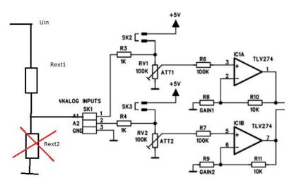
I have chosen not to use the  $R_{ext2}$ . In first instance this might look strange to you, but you need to keep in mind the K8055 circuit already has an internal resistor network. This network is formed by the resistor  $R_3$  and the trimmer  $RV_1$ . Their value are adding up to 101 k $\Omega$ .
